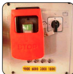
Spindle moulder with 4 rotation speeds
