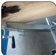
Log holding system
