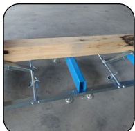
Log holding system
