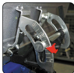
Profiled aluminium guide tilting at 45°
