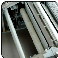
Driving rollers for workpiece feeding
