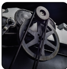
Rollers driven by chain. Double-belt motor drive
