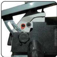
Cast aluminum table tilting at 45°
